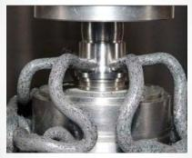
Shown is media being extruded from the lower media cylinder up and out the intersecting holes. With simple fixturing/tooling, the media will surround the part and travel to the upper cylinder and then back
