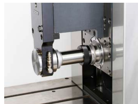
Head mounted diamond roll dressing unit
